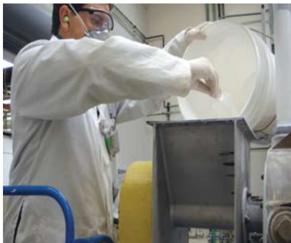
A nanoparticle production worker wearing a personal air sampler and hearing, respiratory, and dermal protection during a pouring operation.
